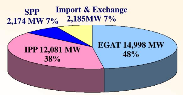
**Total Capacity 31,451 MW** Peak Demand 26,774 MW Load Factor (Max) 83% Load Factor (Avg.) 75%
